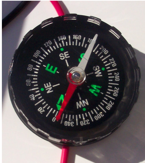
Figure 3 – Compass Needle Deflected When Current is Removed
